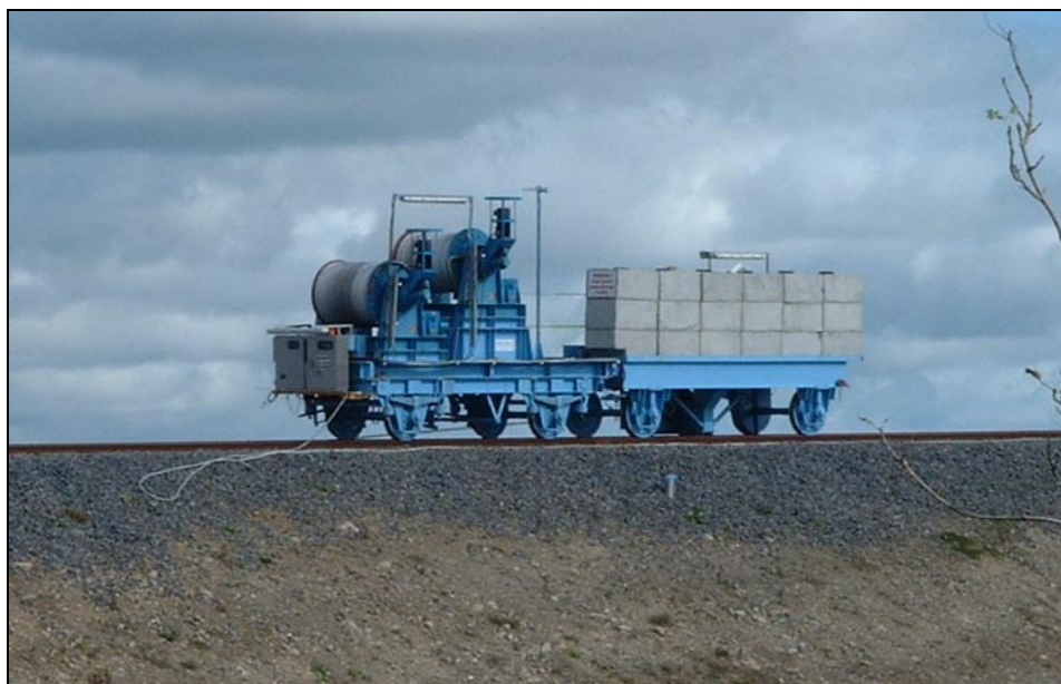
Figure 3.21: Electrically driven winch controlling the tailings distribution pipeline at the Lisheen TMF
